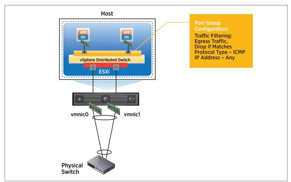
As shown in Figure 10, the traffic-filtering configuration is at the port group level.
